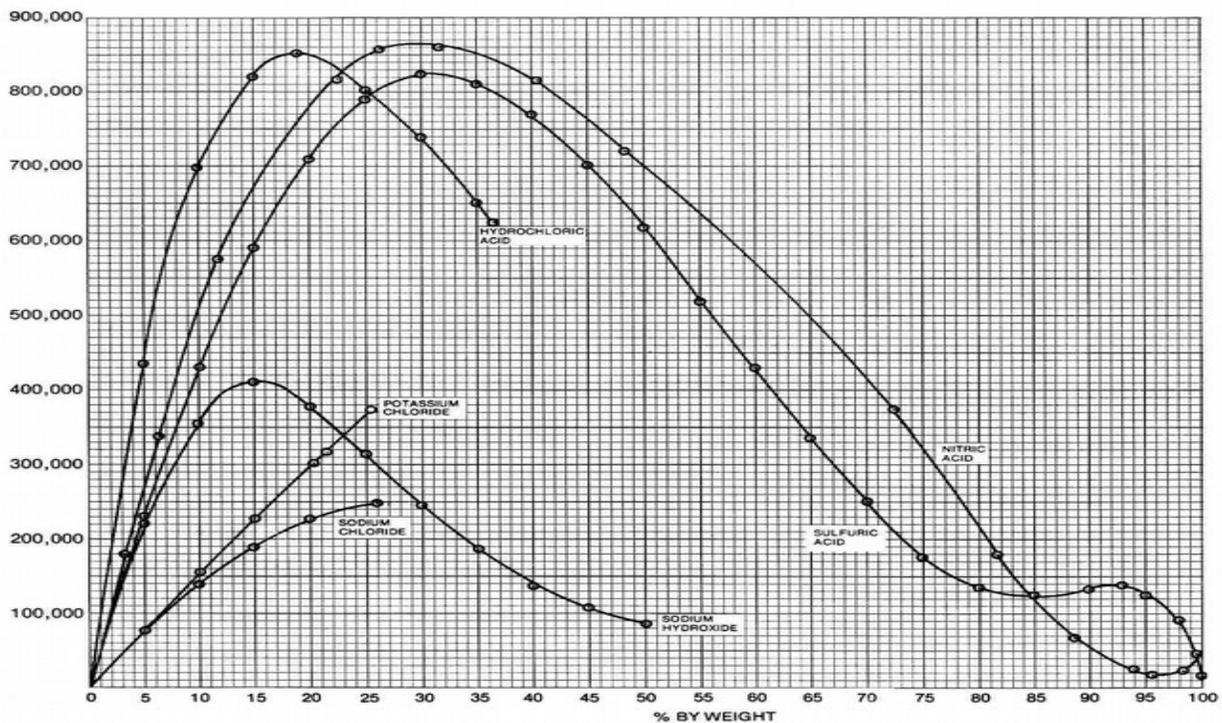
Illustration 1: Conductivity ( $\mu\text{S}/\text{cm}$ ) vs. Chemical Concentration
