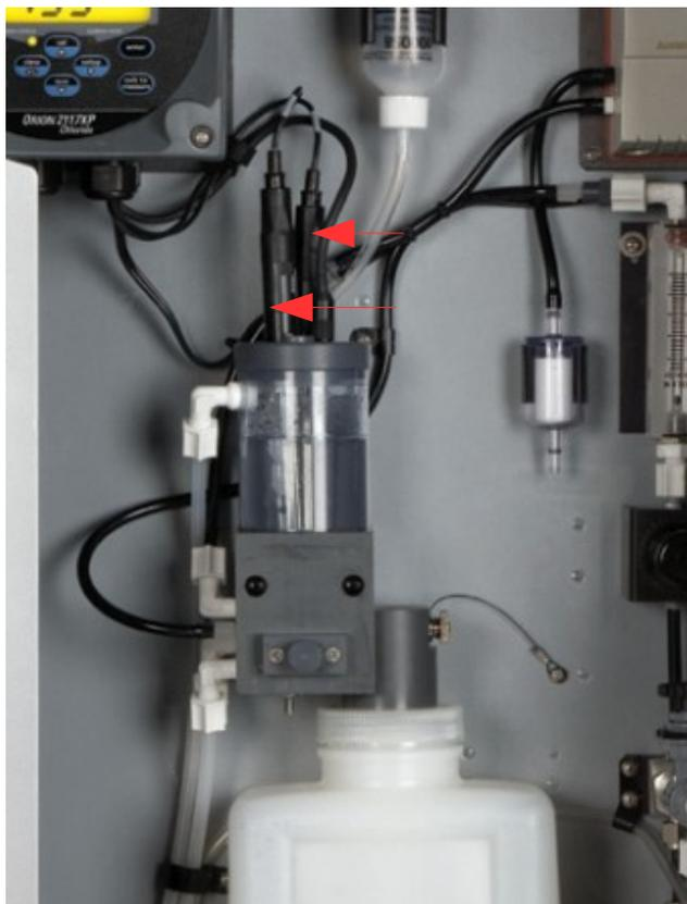
**Figure 2:** Continuous-mode analyzers such as electrochemical sodium monitors use electrodes (indicated by red arrows) in constant communication with a flowing sample
