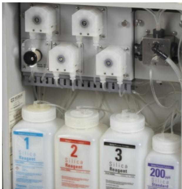
**Figure 1: Batch Analyzers such as those for silica require time to mix the sample with reagent to produce a measurement**
