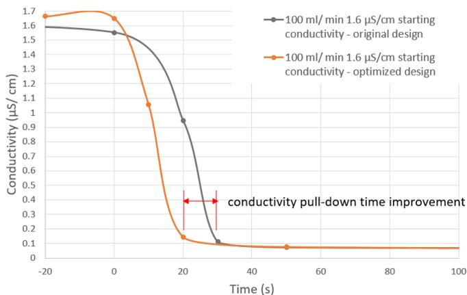
**Figure 3:** Effect of Fluidics Optimization on Sample Stream Stabilization
